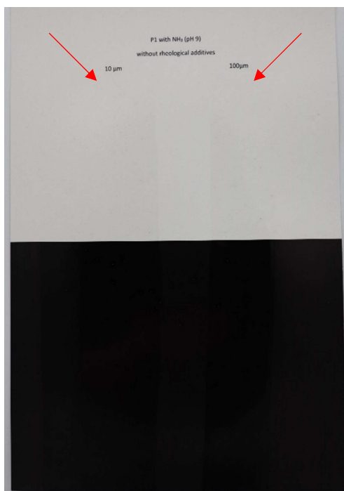
Figure S38. Polymer film of P1c . On the left 10 \mu\text{m} wet film thickness and on the right 100 \mu\text{m} .
