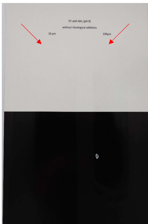
Figure S42. Polymer film of P2c . On the left 10 μm wet film thickness and on the right 100 μm.
