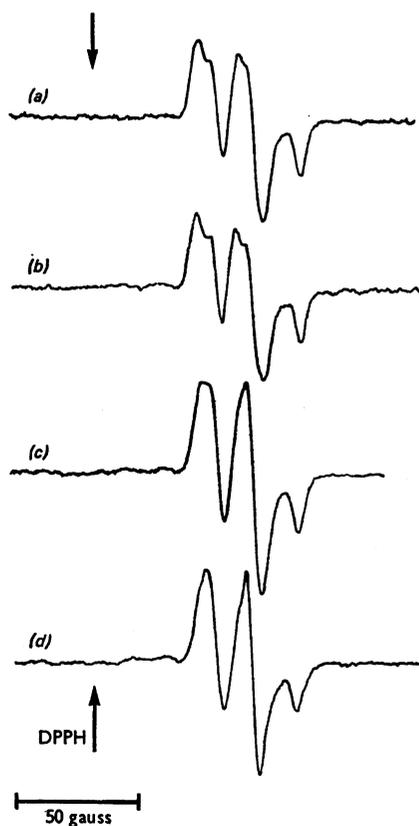
Fig. 5. Variations in the Slowly appearing molybdenum e.p.r. signal, obtained by reducing xanthine oxidase with dithionite, produced on subsequent addition of substrates. The enzyme (0.23 mm final concn.) was treated at pH 8.2 for 1 min. with sodium dithionite (approx. 20 mol.prop.), then with substrates (5 mol.prop.) for 30 min. at 25°, before freezing and recording the 9 GHz spectra at about -150°. The substrates used were: (a) none; (b) salicylaldehyde; (c) purine; (d) xanthine.
