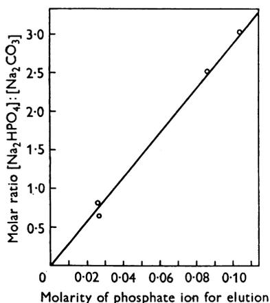
Fig. 6. Chromatography of kidney alkaline phosphatase on calcium phosphate columns. Variation of phosphate ion concentration necessary for elution of the enzyme with  $R=1$ , with the molar ratio  $[\text{Na}_2\text{HPO}_4]:[\text{Na}_2\text{CO}_3]$  in the eluent.
