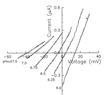
FIGURE 4 pH dependence of the current-voltage relationship of an oocyte expressing the Rostock subtype  $M_2$  protein. The amantadine-sensitive currents were determined at six values of extracellular pH between 6.0 and 7.5. The measurements were begun at pH 7.5 and the changes were reversible. Note the increase in conductance and shift in reversal voltage to more positive values at the lower pH.
