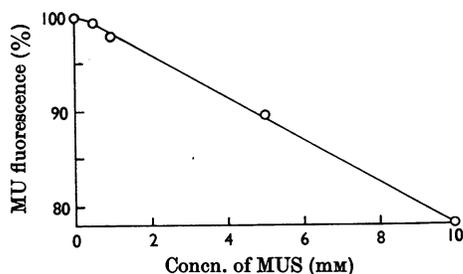
Fig. 1. Filter effect of MUS on the fluorescence of 0.3  $\mu$ M-MU at pH 10.3. Samples were measured with a filter fluorimeter as described in the Materials and Methods section. The fluorescence of MU in the presence of 0-0.5 mm-MUS is  $100 \pm 1\%$ .
