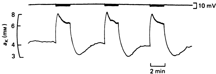
Fig. 9. Recordings from an extracellular site in the superfused retina made with a double-barrelled potassium micro-electrode. The active barrel contained a potassium-selective ligand solution based on valinomycin. The upper trace is the electrical response to photostimulation with trains of flashes. The lower trace is the potassium signal. Because of its high resistance, the response time of the electrode was slow. Because of its high selectivity for potassium over sodium, the relation between potassium signal and \log(a_K) is linear to lower concentrations than is the case for a potassium electrode made with Corning resin 477317. Hence, the potassium signal undershoots the baseline at the end of the stimulation more markedly than in recordings made with the usual electrode as, for example, in that shown in Fig. 6B.
