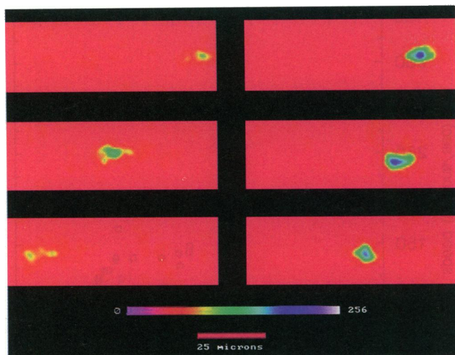
FIGURE 5 False-color fluorescence image of two different cells moving through a common array area. The time between frames is 0.5 s. There is no smearing of the image in this photo because the phosphor decay time of the camera is under 1/30 of a second.
