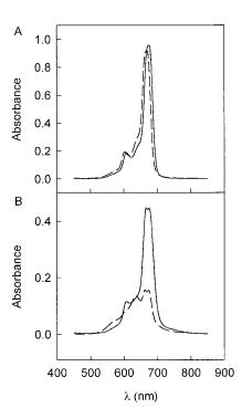
FIGURE 10 The absorption spectra of 5  $\mu$ M AlPcS<sub>4</sub> (A) and 5  $\mu$ M AlPcS<sub>1</sub> (B) in vesicle suspension that contains 20 mM KCl (*spline line*) or 10 mM KCl and 10 mM NaF (*dashed line*). The final lipid concentration was 0.05 mg/ml.
