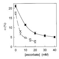
FIGURE 4 The dependence of the relative amplitude of gramicidin photoinactivation ( $\alpha$ , mean  $\pm$  SD, %) on the concentration of ascorbate at the *cis* side ( $\bullet$ ) and *trans* side ( $\bigcirc$ ) of the BLM. AIPcS<sub>3</sub> (1.3  $\mu$ M) is added at the *trans* side of the BLM.  $I_0$  is  $\sim$ 1.5  $\mu$ A.
