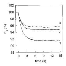
FIGURE 9 The time course of the decrease in the gramicidin-mediated current (*I*) across the BLM after a flash of visible light (at t=0 s) in the presence of 0.16  $\mu$ M AlPcS<sub>1</sub> at the *trans* side of the BLM (*curve 1*,  $\alpha_1=8.3\%$ ,  $\tau_1=1.43$  s). *Curve 2*: The addition of 3 mM NaF at the *trans* side of the BLM ( $\alpha_2=5.3\%$ ,  $\tau_2=1.22$  s). *Curve 3*: The addition of 10 mM NaF at the *trans* side of the BLM ( $\alpha_2=4.4\%$ ,  $\tau_2=1.14$  s).
