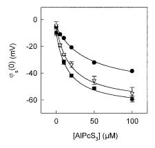
FIGURE 12 Surface potential  $\varphi_s(0)$  of large unilamellar DPhPC vesicles as a function of AlPcS<sub>3</sub> concentration. With an increase of the ionic strength from 10 mM KCl to 20 mM KCl, and finally to 100 mM (*from the bottom to the top*), the electrophoretic mobility and hence  $\varphi_s(0)$  decreased.
