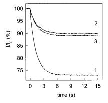
FIGURE 3 The time course of the decrease in the gramicidin-mediated current (I) across BLM after a flash of visible light (at t=0 s) in the presence of 1.3  $\mu$ M AlPcS $_3$  at the cis side of the BLM ( $curve\ I$ ), 1.3  $\mu$ M AlPcS $_3$  at the cis side and 13  $\mu$ M AlPcS $_3$  at the trans side of the BLM ( $curve\ I$ ), and 13  $\mu$ M AlPcS $_3$  at the trans side of the BLM (trans side of the
