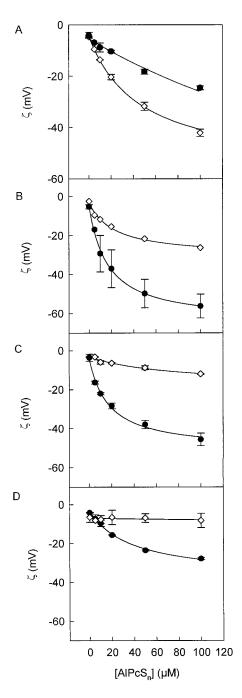
FIGURE 8 The ζ-potential of large unilamellar DPhPC vesicles as a function of photosensitizer (A: AlPcS<sub>1</sub>; B: AlPcS<sub>2</sub>; C: AlPcS<sub>3</sub>; D: AlPcS<sub>4</sub>) concentration in 20 mM KCl ( $\bullet$ ) or 10 mM KCl and 10 mM NaF ( $\diamondsuit$ ) in the buffer solution. The ζ-potential was calculated from vesicle electrophoretic mobility.
