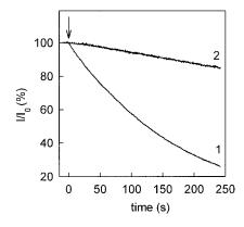
FIGURE 6 The kinetics of the decrease in the gramicidin-mediated current (I) across the BLM induced by illumination with a He-Ne laser (30 mW/cm<sup>2</sup>) in the presence of 1.3  $\mu$ M AlPcS<sub>3</sub> at the *trans* side of the BLM (*curve 1*), and 1.3  $\mu$ M AlPcS<sub>3</sub> and 10 mM NaF at the *trans* side of the BLM (*curve 2*).  $I_0=1.0~\mu$ A. The illumination is switched on at the moment marked by an arrow.
