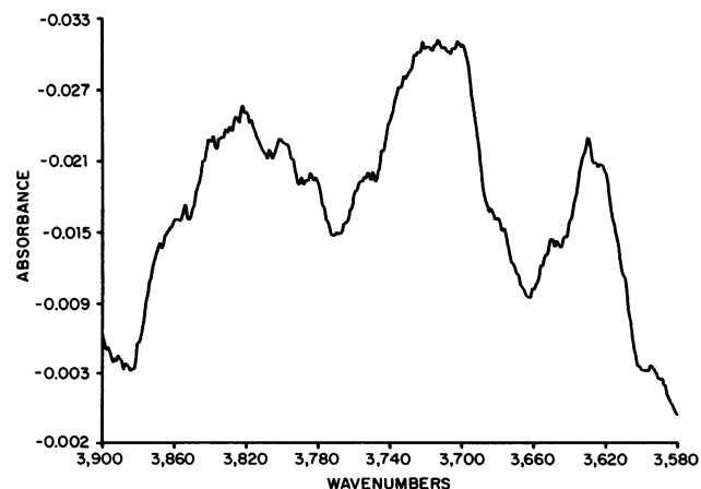
FIGURE 4 The infrared spectrum of the OH stretching region of water in n -tetradecane taken under the same conditions as that of Fig. 1. The absorbance scale has been multiplied by 10. The solvent has a weak band at \sim 3,630 and the band seen at about this position of our water spectrum may result from imperfect subtraction of the solvent band.
