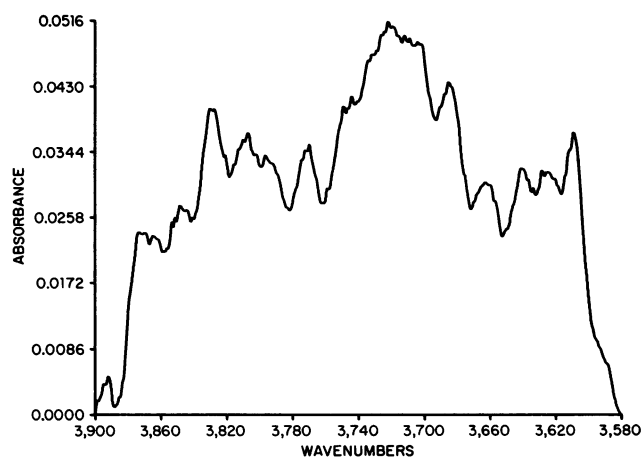
FIGURE 3 The infrared spectrum of the OH stretching region of water dissolved in n -undecane taken under the same conditions as that of Fig. 1. The absorbance scale in the figure has been multiplied by 10.
