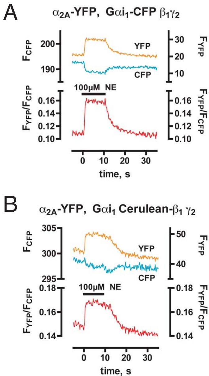
(A) Agonist-dependent FRET signal of cells transfected with  $\alpha_{2A}$ -YFP and G $\alpha$ i<sub>1</sub>-CFP  $\beta_1\gamma_2$ . (B) Agonist-dependent FRET signal of cells transfected with  $\alpha_{2A}$ -YFP and G $\alpha$ i<sub>1</sub>Cerulean- $\beta_1\gamma_2$ .
