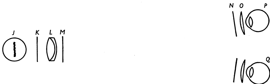
Text-fig. 1. Diagram of apparatus in plan. J : 48 W 12 V car headlamp bulb. K : camera shutter. L : lens forming an image of the filament of J on P and Q . M : colour filter or grating. N : colour filter. O : spectacle lens. P and Q right and left eyes of subject.
