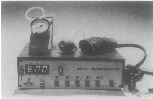
Figure 1 Front view of the Auto-Manometer. The air inlet, and an outlet for connection to a mercury manometer for calibration are on the back. The cuff inlet is on the right side. The lever to the left is used to determine inflation pressure level. When the inflation-deflation switch is flicked to inflation, INF lights up in the display window. Inflation pressure is increased manually whilst Korotkov sounds are auscultated, and when systolic level has been surpassed, the switch is flicked to deflation; DEF then lights up in the display window.
