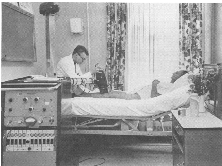
FIG. 1. View of detection system consisting of a scintillation probe, pulse height analyzer and scaler, mounted on mobile stand. Seven counting areas marked off on each leg from the ankle to the groin. Patient lies comfortably in bed.
