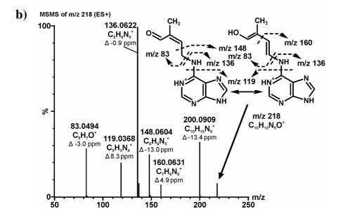
Supplement 2 MS/MS analysis of ZmCKX1 (1.5  $\mu$ M) reaction with cytokinins: (a) *trans*-zeatin (50  $\mu$ M), (b) *trans*-zeatin[-2H] intermediate.
