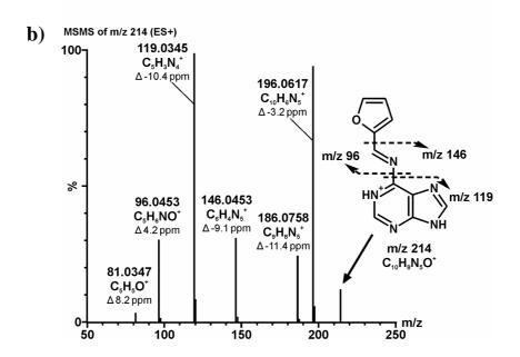
Supplement 3 MS/MS analysis of ZmCKX1 (1.5  $\mu$ M) reaction with cytokinins: (a) kinetin (50  $\mu$ M), (b) kinetin[-2H] intermediate.
