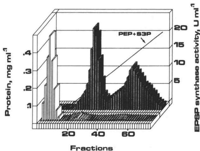
**Figure 1.** Purification of EPSP synthase from the BMS cell line. Substrate-elution chromatography on a phosphocellulose column that was equilibrated at pH 6.0. Fraction volume = 2.5 mL. Sample elution with a linear gradient of both the substrates of EPSP synthase (PEP and S3P) resulted in two well-separated enzyme activities.
