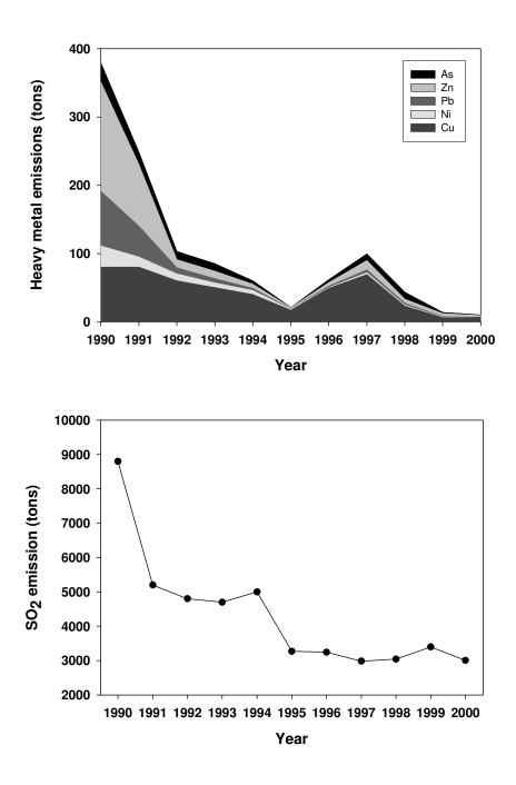
**Appendix I**. Heavy metal and SO<sub>2</sub> emissions from the Harjavalta copper smelter in 1990 - 2000. In 1994, a new 140 m high stack came on line in the smelter complex together with more effective filters. As a result emissions decreased and were spread farther from the smelter. Increased copper production and problems with filters again increased heavy metal emissions in 1996-1997. Data from Harjavalta copper smelter.
