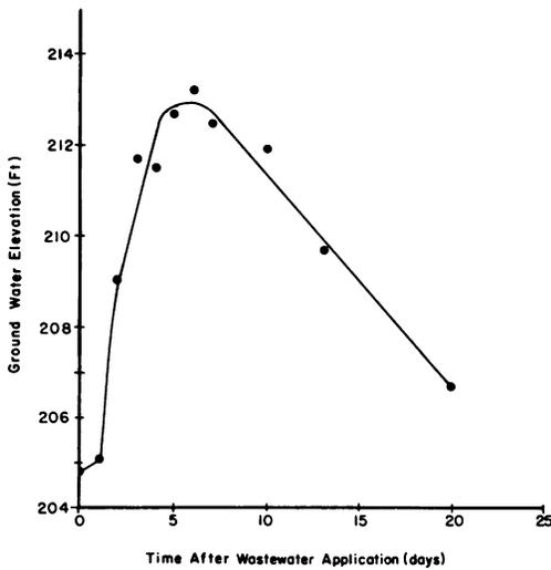
FIG. 4. Groundwater mound at observation well directly beneath wastewater application zone. Observation well 15 was observed for groundwater mounding with a measured conductivity probe for 21 days after testing was initiated.
