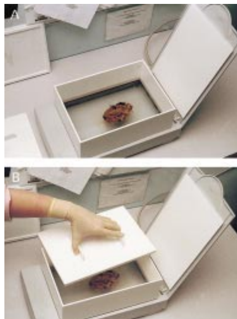
Figure 1 (A) The perspex box mounted on the scanner. (B) Application of the heavy sliding insert.
