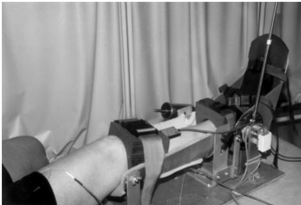
Figure 1 Photograph of the ankle rig showing the position of the leg, electrodes, potentiometer, strain gauge, counterbalance, and lever.
