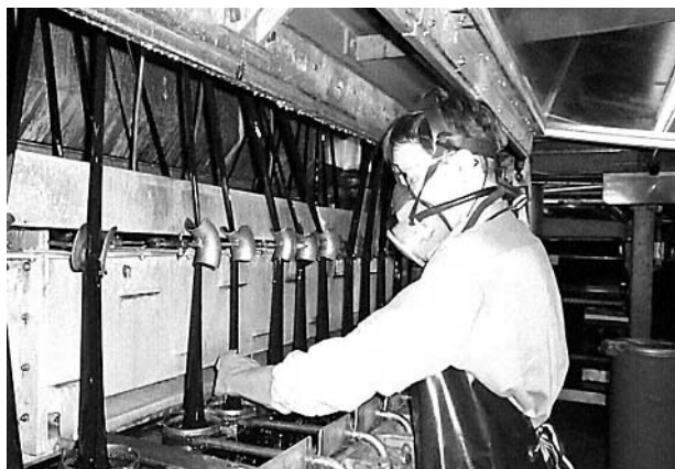
Figure 2 Manually starting the spinning process. Chemical resistant clothing, breathing masks, and non-permeable gloves are required.
