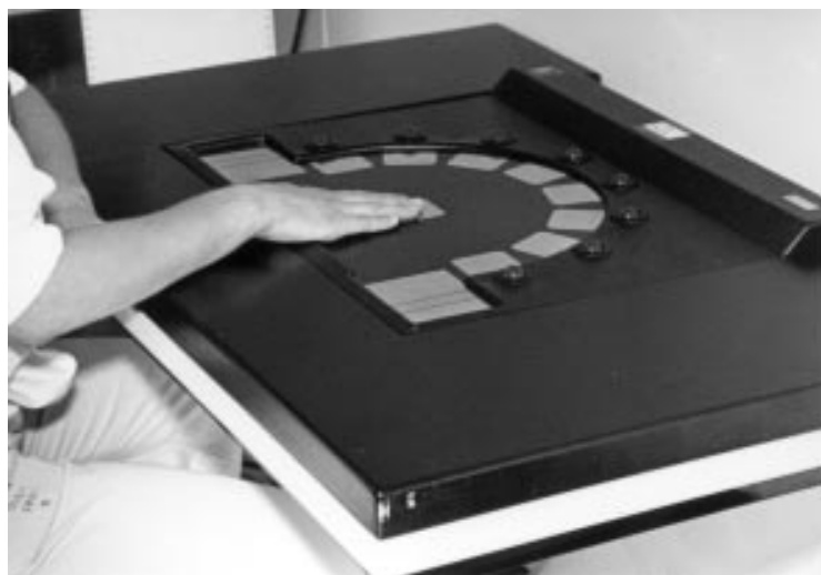
Figure 1 Human Performance Measurement/Basic Elements of Performance device and the measurement of reaction time of the hand.
