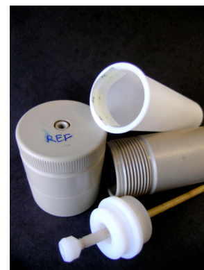
Fig. S3 Example of reaction format used for “blanket-type” MW reactions on planar supports. A planar cellulose array can be seen in the Teflon sheath (white) that will be placed inside the PEEK vessel (brown).
