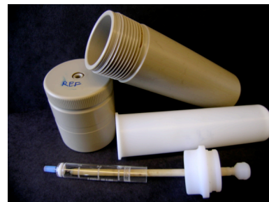
Fig. S4 Example of reaction format used for MW-assisted reactions performed on beads. The beads are placed in a glass synthesis vessel and then placed inside a Teflon/PEEK MW reaction vessel.
