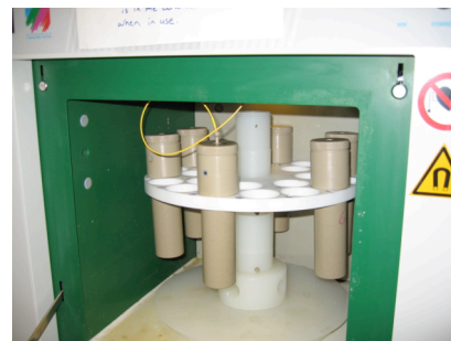
Fig. S1 View of the inside of the Milestone MicroSYNTH reactor showing the rotor and the 70 mL Teflon/PEEK reaction vessels. The yellow cord is the fiber-optic temperature sensor.
