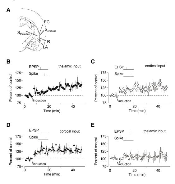
(A) A schematic representation of the experimental design that shows the position of the recording (R) and stimulation (S) electrodes. EC, external capsule. (B) Summary graph of the LTP experiments in thalamic input without PTX in the bath solution at room temperature, when postsynaptic neuron was depolarized to -20 mV during the induction (n = 8). To induce LTP, 80 EPSPs were evoked at a frequency of 2 Hz; each EPSP was paired with action potential induced
