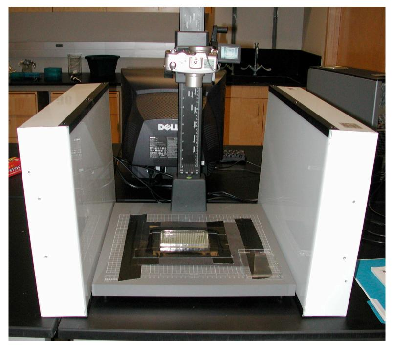
Shown are the digital camera, camera stand, and lighting sources assembled for image capturing.
