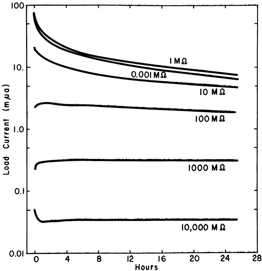
Graph 1. Current levels obtained from silver-platinum couplings with various levels of interposed resistors. Measurements were made *in vitro* with a Hewlett-Packard 425A microvolt ammeter with electrodes immersed in normal mammalian saline. Not only is the steady state current altered by the resistor, but the initial current drop is markedly changed as well.
