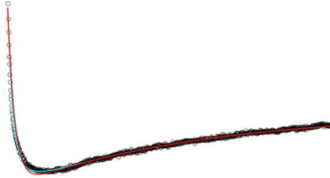
SI Fig. 8. Comparison of the experimental data (open circles), the fit of the data with a triple exponential function (blue line), and the modeled double exponential fit (red line).
