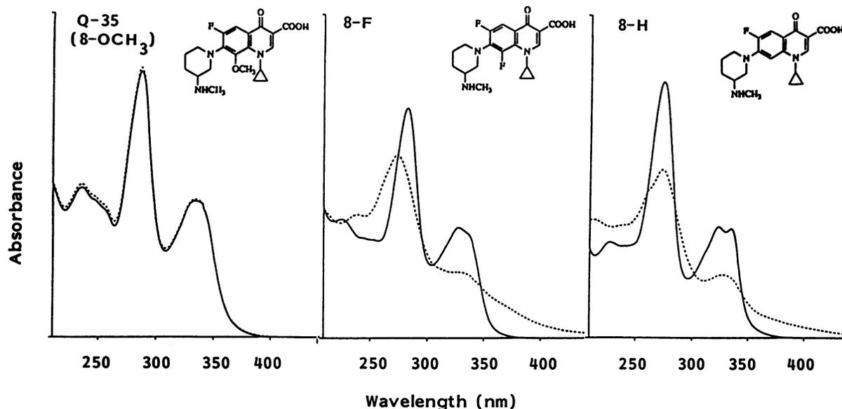
FIG. 1. Change in UV absorption spectra in the solution of 8-substituted fluoroquinolones. Forty milliliters of the solution containing 20  $\mu\text{g}$  of each fluoroquinolone per ml was transferred to a 50-ml beaker, which was stirred with a magnetic bar, and the solutions were irradiated with 3 J of UVA per  $\text{cm}^2$ . The absorbances of preexposure (—) and postexposure (---) solutions were determined with a UV spectrophotometer.
