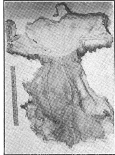
FIG. 2.—This ballet frock, belonging to a child aged 6, caught fire owing to contact with a gas-ring on the floor. The flared skirt, which was made of cambric and cotton net, was extensively destroyed, and analysis showed that the vertical flame-speed over these fabrics was 1 ft. (30 cm.) per sec. The more closely fitting bodice made of wool, satin, and acetate rayon was much less extensively burnt.
