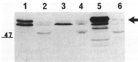
FIG. 12. Anaerobic induction of HYD1. Western analysis of extracts from wild-type cells (TG1, lanes 1 and 2), AP1 cells (lanes 3 and 4), and AP1 cells complemented with pCL47 (lanes 5 and 6), grown either anaerobically (lanes 1, 3, and 5) or aerobically (lanes 2, 4, and 6). The arrow indicates HYD1.
