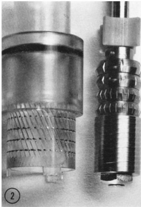
FIGURE 2 Lower end of continuous dissector: (left) stationary part, showing the grooved sleeve with three or four rows of needles protruding into the grooves; (right) rotating part with transporting cylinder, four squeezing discs and one of the plastic spacers that center the rotating part within the stationary part during operation.
