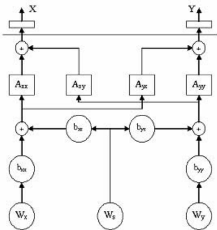
Figure A1. Linear generation model of signals  $X$  and  $Y$
