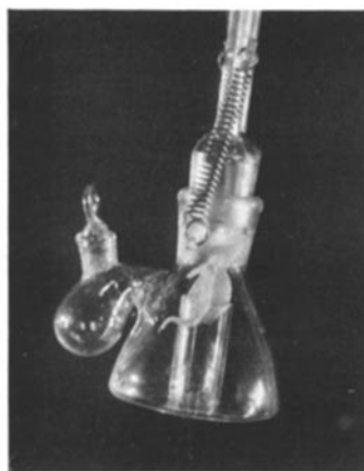
FIG. 1. A castor bean with well developed hypocotyl inside the respirometer bottle resting on top of the well.
