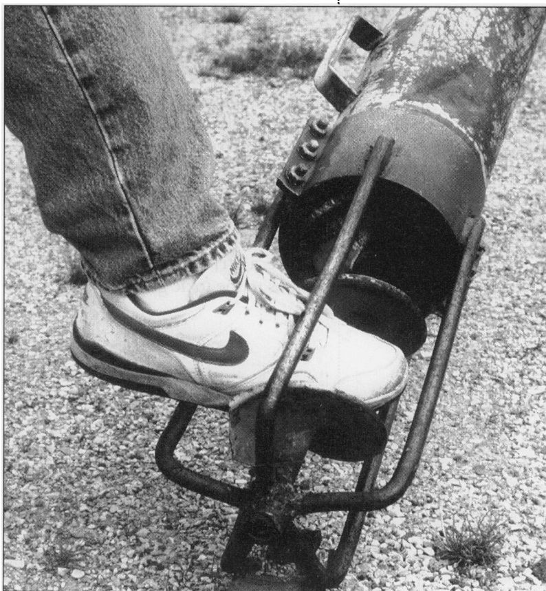
Figure 5. Safety screens are often removed from grain augers, increasing the risk that a limb will become caught in the mechanism.
