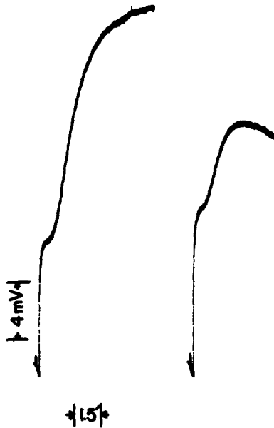
FIGURE 8. The time course of the potential following a change from 0.03 M NaCl to 0.5 M NaCl (left) and a change from 0.03 M NaCl to 0.5 M KCl (right). The second component is always greater for NaCl. This particular result was obtained with saturated KCl salt bridges.
