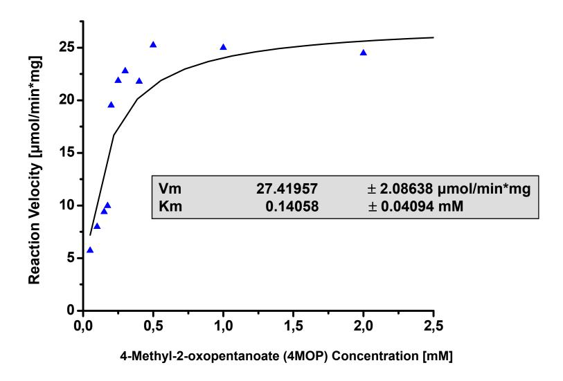
Reaction velocity is plotted against ketoisocaproate concentration. The data were fitted into a non-linear regression, which allows the calculation of the above mentioned  $V_{\text{max}}$  and  $K_{\text{m}}$  values.
