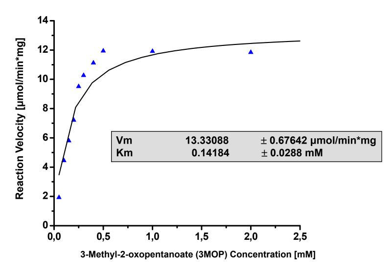
Plotting of reactions velocity against methionine concentration revealed that BCAT3 shows Michaelis-Menten kinetics. The above mentioned Vmax and Km values are calculated by fitting the data into a non-linear regression.
