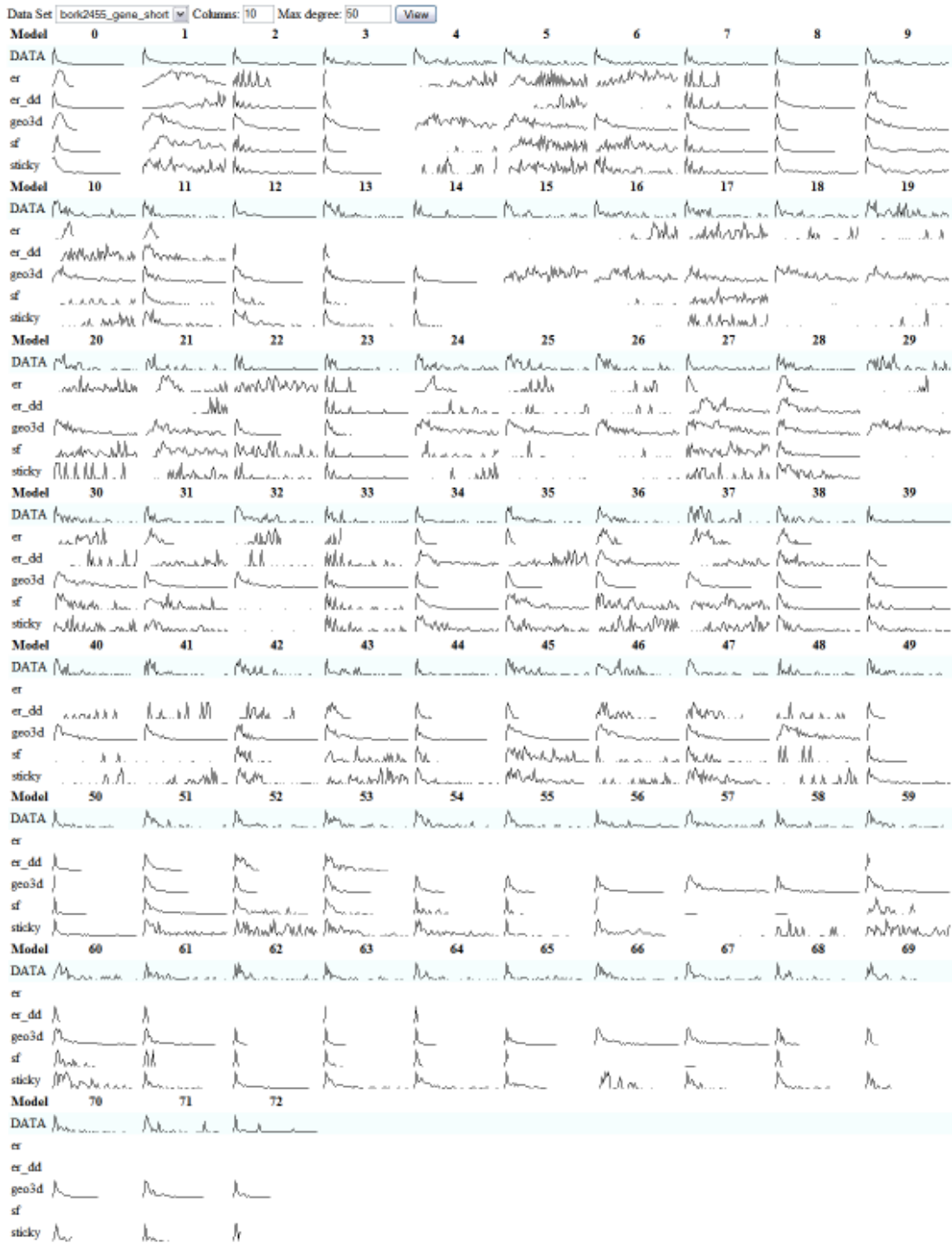
Figure S6. GDD Viewer page of the GraphCrunch on-line web user interface. It contains plots of graphlet degree distributions (GDDs) for each of the 73 orbits of real-world and model networks. In the figure, GDDs of the data set named “bork2455_gene_short” (denoted by “DATA” and highlighted in blue) and five model networks (denoted by “er”, “er_dd”, “geo3d”, “sf”, and “sticky”) are shown. The plots illustrating ten GDDs are displayed in each row, and 50 is chosen to be the maximum degree on x-axis in each of the plots.
