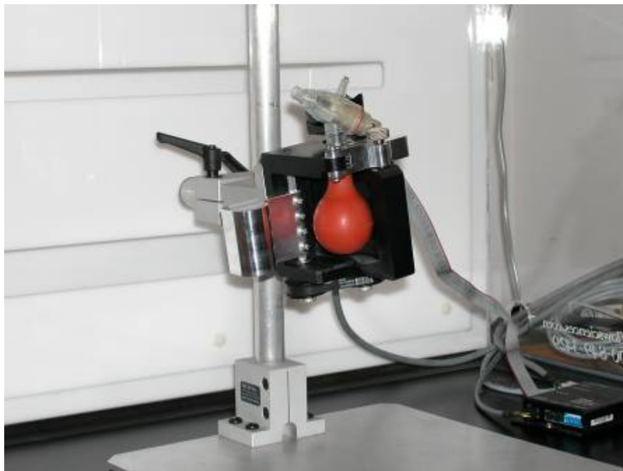
SI Fig. 6. Newborn dry powder inhaler device with in vitro actuation system.
