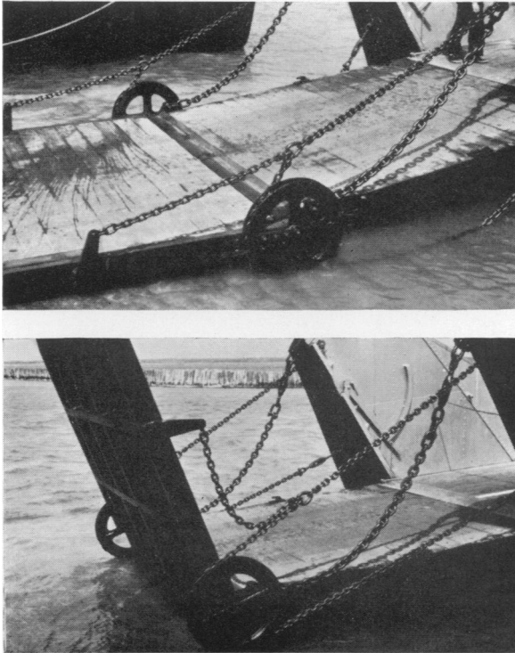
Fig. 2. The ramp of this car ferry is let down in two parts. The chain which pulls it up and lets it down has two attachments. One operates in flexion of the distal joint and the other in extension.
