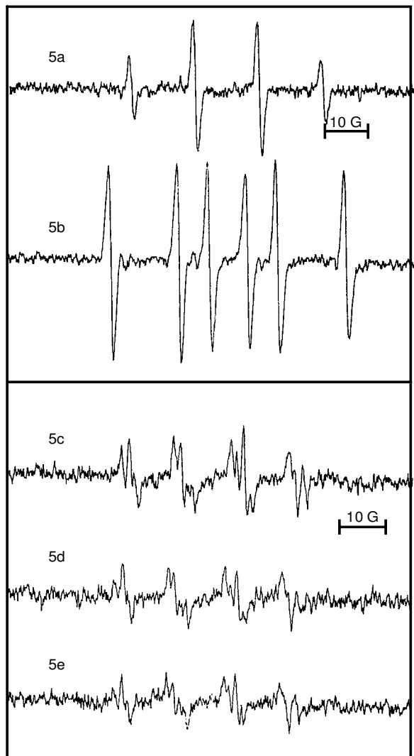
FIG. 5. ESR spectra (DMPO 100 mM) of the spin adduct of hydroxyl radical generated by the Fenton reaction [ H_2O_2 (88 mM), Fe^{2+} (0.01 mM), EDTA (0.01 mM)] (a and b) and superoxide spin adduct generated by xanthine (50 mM)/xanthine-oxidase (110 mU/ml) system in HBSS buffer pH 7.4 (c, d and e). (a) Normal spectrum (hyperfine splittings for DMPO·OH: a_H = a_N = 14.87 G). (b) Same as 5a + 1% ethanol: the spectrum of the DMPO-ethoxy adduct is observed (hyperfine splittings for DMPO·C(CH 3 )OH: a_H = 15.67 G, a_N = 23.0 G). (c) Complete system xanthine/xanthine-oxidase generating superoxide radical, in the presence of DMPO, without SPN. (d) Complete system in the presence of 4 \times 10^{-6} M SPN. (e) Complete system in the presence of 8 \times 10^{-6} M SPN.
