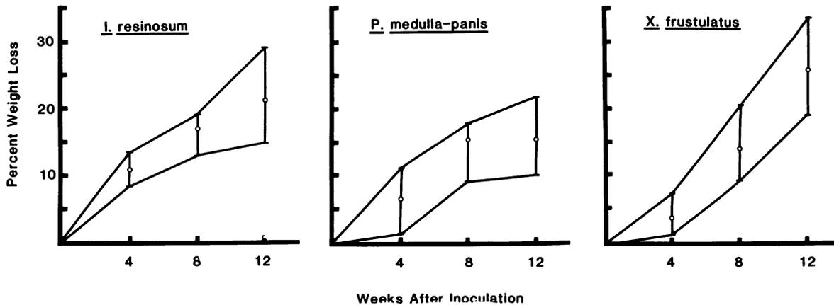
FIG. 4. Percentages of weight loss in aspen blocks caused by *I. resinosum*, *Poria medulla-panis*, and *X. frustulatus* after 4, 8, and 12 weeks. Circles indicate mean values, and bars represent ranges.
