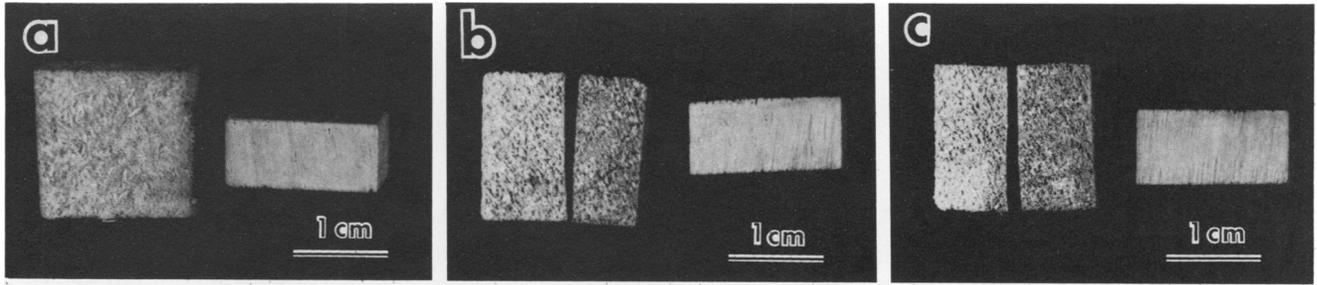
FIG. 1. Tangential and radial sections of wood blocks decayed for 4 weeks by *I. resinosum* (a), *Poria medulla-panis* (b), and *X. frustulatus* (c).
