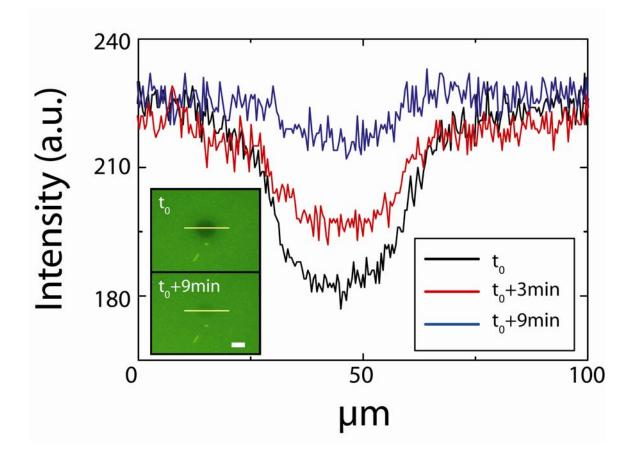
Supplementary Figure 4 Lateral mobility of Ras-coupled supported lipid bilayers. Membrane-linked Ras mobility is detected by fluorescence recovery after photobleaching (FRAP) experiments. High intensity illumination is used to bleach a small region of the membrane, bleaching most of the BODIPY-GDP fluorophores. After 9 minutes the bleached fluorophores have laterally diffused out of the spot, as indicated by intensity traces along the yellow line. [White bar =  $20 \mu m$ ]
