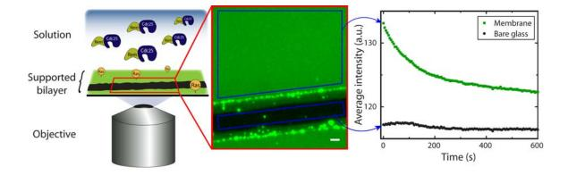
**Supplementary Figure 5** Schematic of supported lipid bilayer experimental setup. A planar bilayer in a 400  $\mu$ l well presents mobile, lipid-linked Ras to the solution (left). A small region of bilayer is removed by scratching with a needle (center, bar = 100  $\mu$ m). Upon addition of SOS, signal from the bilayer decays with time, while the scratched region controls for signal from fluorescent nucleotide in solution (right).
