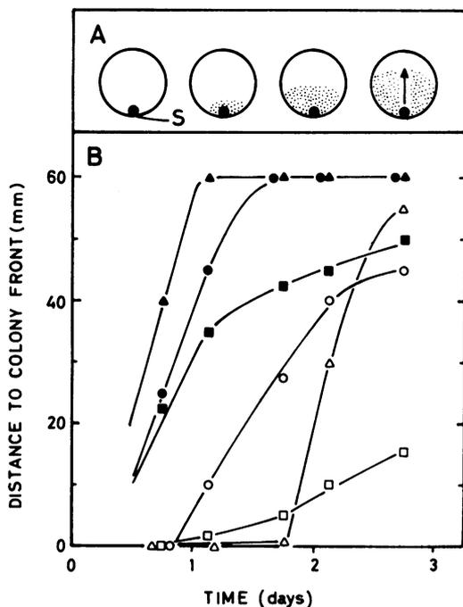
FIG. 3. Substrate gradient test of the growth of CP 366 and CP 367 with different substrates. (A) Schematic presentation of the substrate gradient test. S, substrate spot. The small dots indicate colonies which, as incubation is prolonged, become visible at increasing distance (arrow) from S. (B) Progression of the colony front (as distance from the substrate spot) with time of wild-type CP 366 (filled symbols) and CP 367 (open symbols) with glucose (O), lactose (□), or proline (Δ) as substrate.
