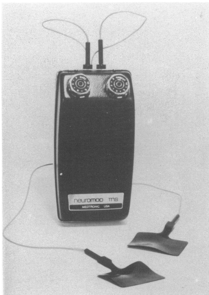
FIG. 3 Modern transcutaneous electrical (neural) stimulator. Two electrode terminals. Hand control of output and frequency.
