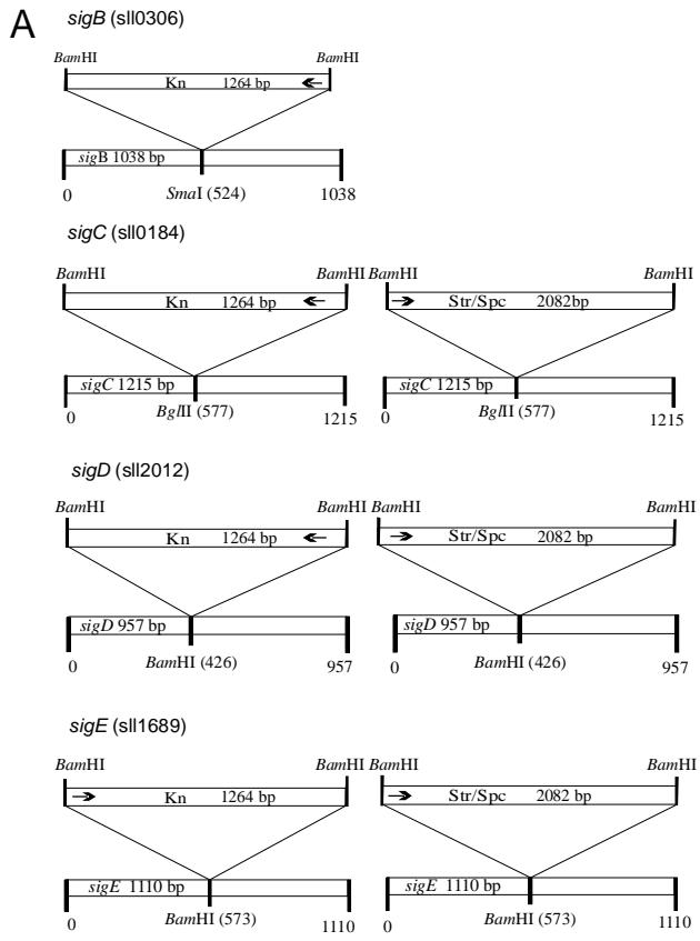
Supplement Figure S1. Sigma factor inactivation strains of *Synechocystis* sp. PCC 6803. Schematic representation inactivation strategies. Arrows indicate the orientation of the antibiotic resistance cassette.
