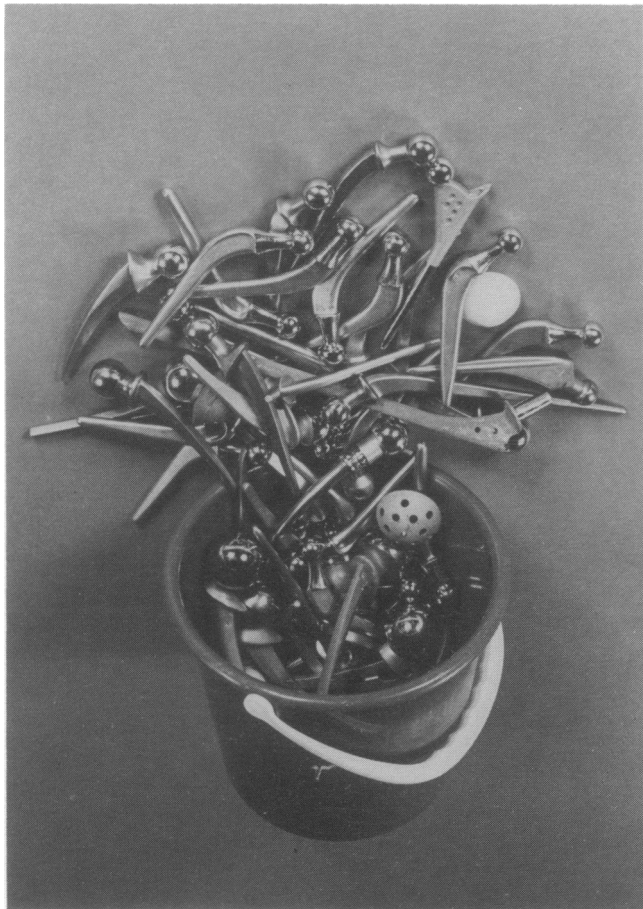
Figure 1. The pile of total hip replacements recently removed at revision surgery from patients in our unit. Each represents a disaster for a patient.
