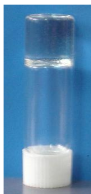
Figure 1: Inverted vial containing a gel of compound 3 in mesitylene (0.65% w/v). Photograph was taken after 4 h of cooling at RT).
