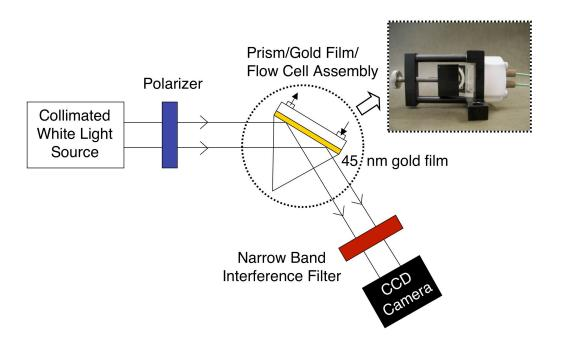
Figure S.1. A simplified schematic diagram of SPR imager.
