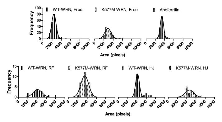
Size Distribution Histograms of Wild-type and K577M-WRN with Calculated Gaussian Curves. The projected areas of free and DNA-bound wild-type and K577M-WRN, and apoferritin were measured from EM images and used to construct frequency distribution histograms. Each histogram was fitted with a Gaussian distribution using GraphPad Prism (version 5) to determine peak values. RF and HJ refer to replication fork DNA and Holliday junction DNA, respectively.
