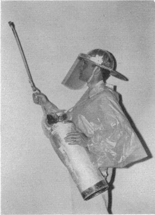
Note the almost complete coverage afforded the arms by this cape. Gloves would ordinarily be used with this equipment.
